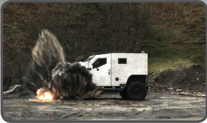
Military vehicle STANAG 4569 blast test
